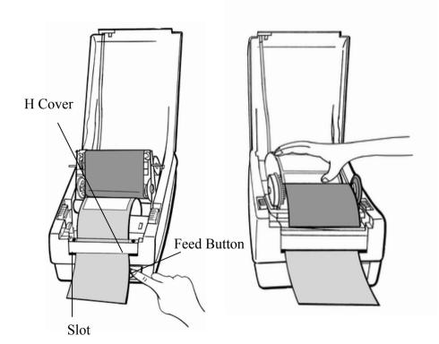
15. Close the top cover and turn on the printer or press the "FEED"
